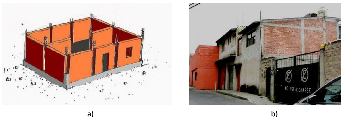
Figure 2.35 Confined masonry construction: a) construction sequence, and b) a confined masonry building in Mexico City, Mexico (Illustrations: a) T. Schacher, and b) S. Brzev)
