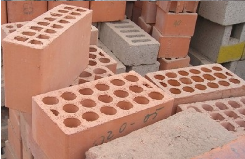
Fired clay hollow bricks with vertical perforations, Peru (S. Brzev)
