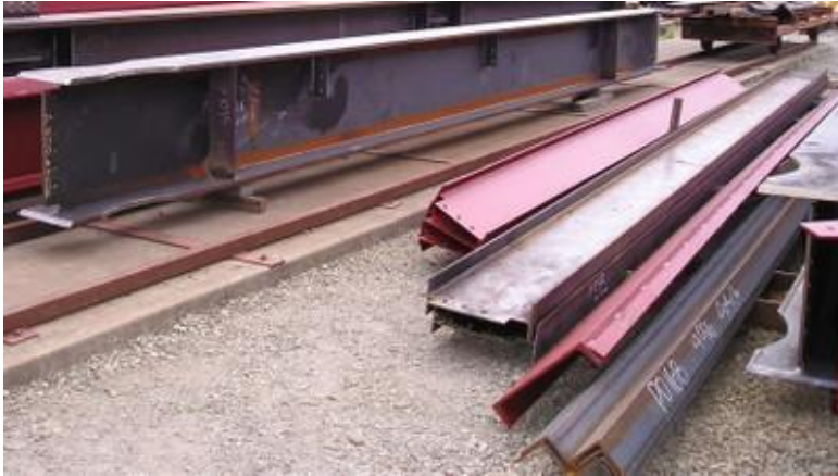
Hot-rolled steel sections at a construction site: I-shaped (called W sections in North America), channel sections (called C sections in North America, etc. (Canada - S. Brzev)
