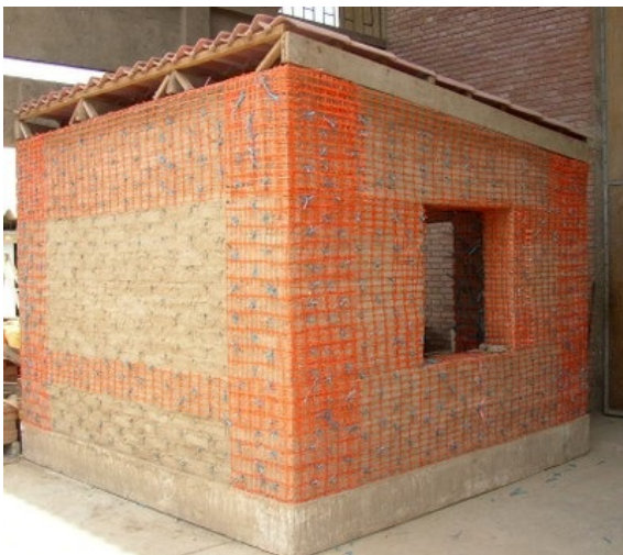
Polymer mesh (geogrid) laid in form of horizontal and vertical bands, adobe walls, Peru (left-S. Brzev and right-N. Tarque)
