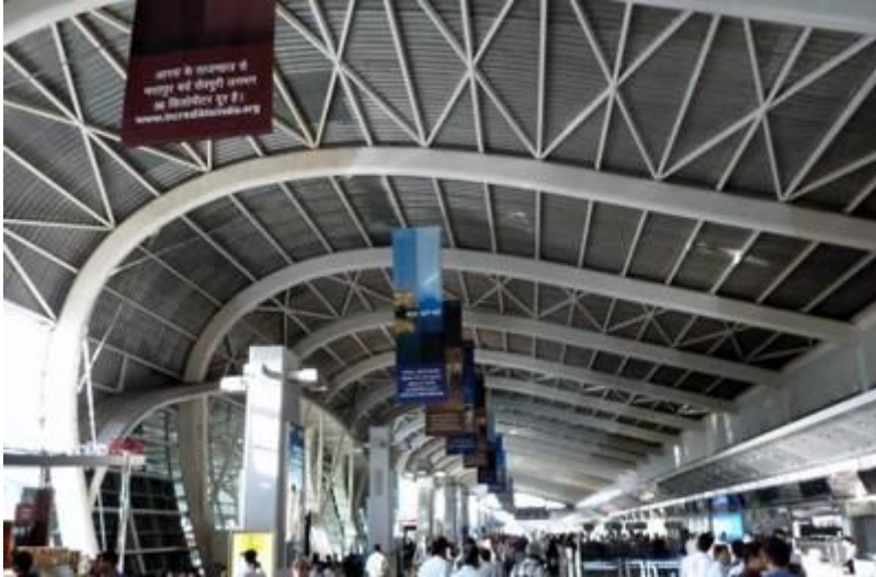
Curved steel beams supporting corrugated steel sheet roofing, Mumbai, India (S. Brzev)
