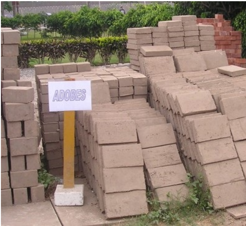
Adobe blocks of different shapes and sizes, Peru (S. Brzev)
