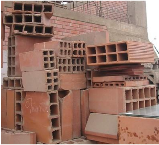
Fired hollow clay bricks with horizontally-laid perforations, Peru (S. Brzev)
