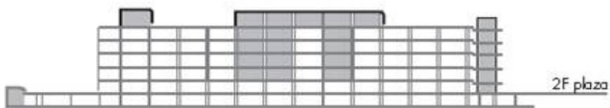
Soft storey in reinforced concrete buildings, India (S. Brzev)
