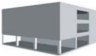
Offset structure - discontinuous shear walls (FEMA 454, 2006)
