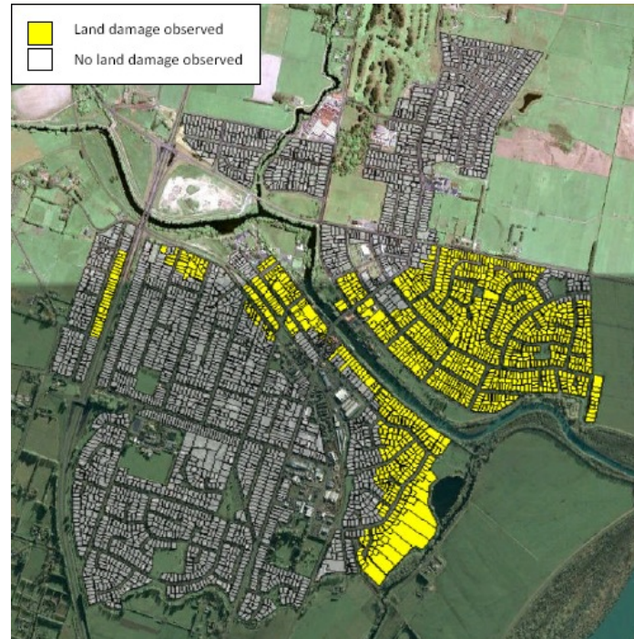
Figure 2.9 Overview map showing extent of observed land damage due to liquefaction in Kaiapoi town, New Zealand due to the September 4, 2010 Darfield earthquake (Source: Tonkin and Taylor (2010))
