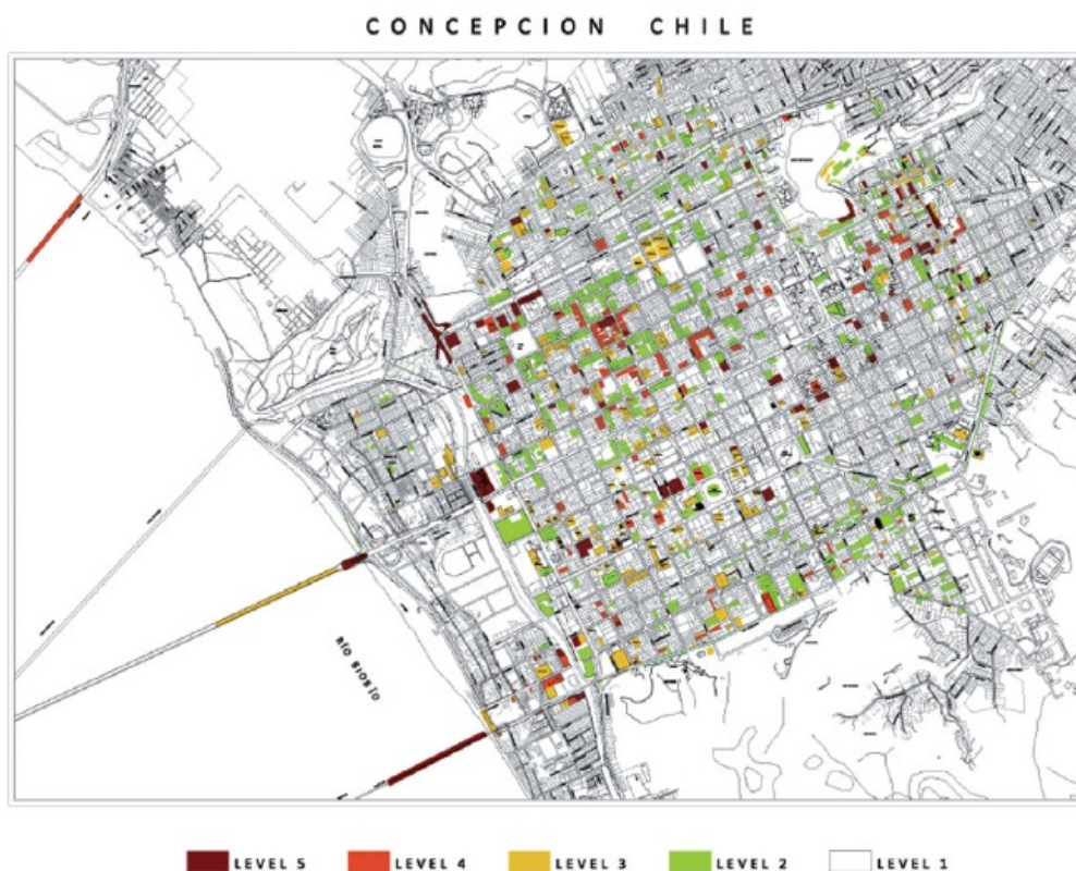
Figure 2.4 Map of distribution of damage to buildings regardless of type of structure, height and age in the city centre of Concepción due to the February 27, 2010 earthquake (Betanzo, 2010)
