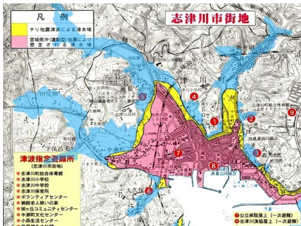
Figure 2.13 Tsunami inundation map of Minamisanriku town (Miyagi prefecture, Japan). This map shows the tsunami flood zone during the 1960 Chile and the 2011 Tohoku tsunami (in yellow and blue respectively). The pink flood zone is the tsunami hazard map compiled for the town authorities prior to the 2011 tsunami based on a more moderate tsunamigenic earthquake ( M_w < 8 ) occurring offshore Miyagi Prefecture's coast.
