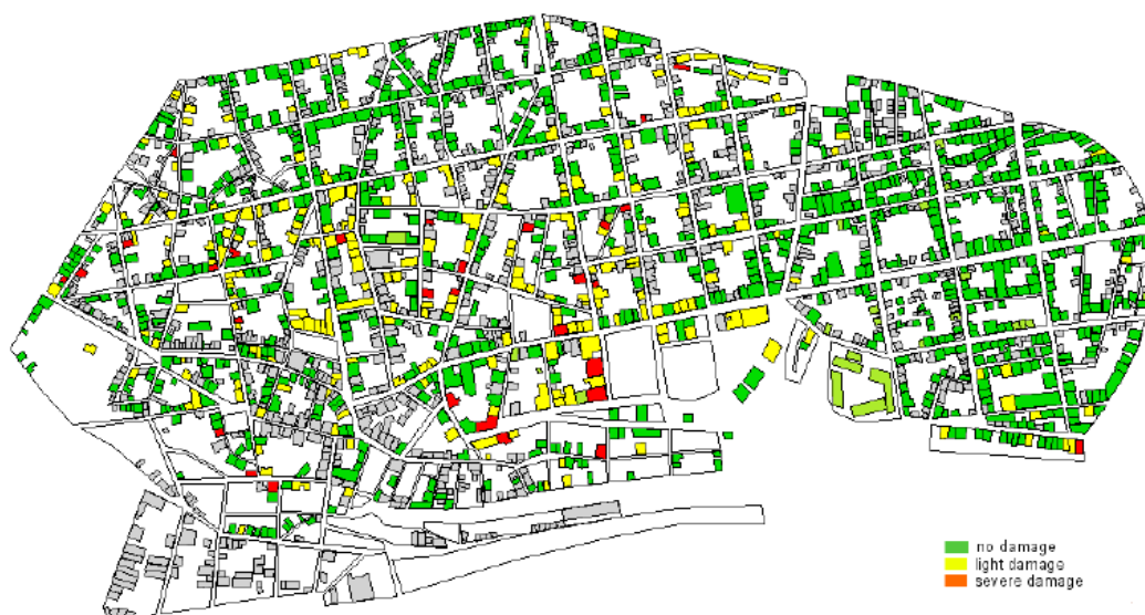
Figure 2.3 Damage survey for RC buildings in the city centre of Aegion city (Greece) affected by the June 1995 earthquake (Karantoni and Fardis, 2004) recorded on a cadastral map. Buildings in grey are unreinforced masonry and have also been surveyed and an equivalent map is shown in Karantoni and Fardis, 2005.
