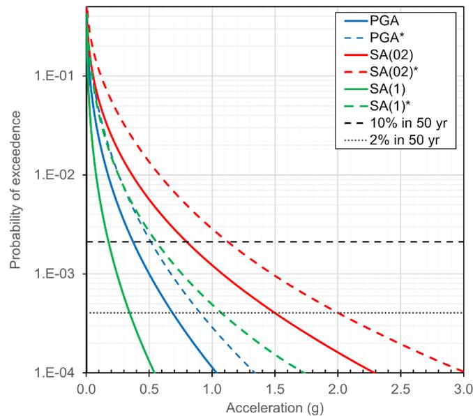
**Figure 14. Hazard curves for Santiago de Cali city. The colored lines indicate acceleration for different structural periods (PGA, SA for 0.2 and 1.0 seconds) for rock condition ( $V_{s30} = 800$  m/s) while dashed colored lines correspond to the same structural periods but referred to soil condition ( $V_{s30} = 160$  m/s) The probability of exceedance (PoE) is for an investigation time of 1 year. Dashed and dotted black lines correspond to 2% and 10% PoE in 50 years respectively.**
