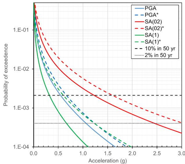
Figure 24. Hazard curves for Quito city. The colored lines indicate acceleration for different structural periods (PGA, SA for 0.2 and 1.0 seconds) for rock condition ( $V_{s30} = 800$  m/s) while dashed colored lines correspond to the same structural periods but referred to soil condition ( $V_{s30} = 320$  m/s) The probability of exceedence (PoE) is for an investigation time of 1 year. Dashed and dotted black lines correspond to 2% and 10% PoE in 50 years, respectively.
