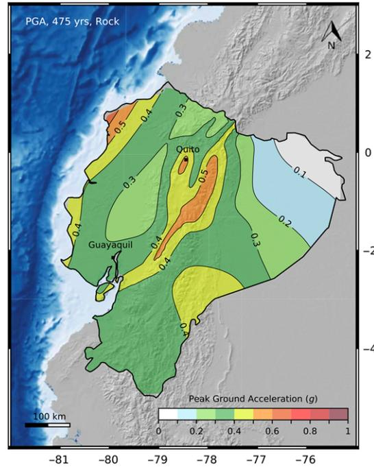
Figure 18. –. Mean PGA with 10% probability of exceedance in 50 years proposed by Beauval et al. (2018). Source: Beauval et al. (2018)
