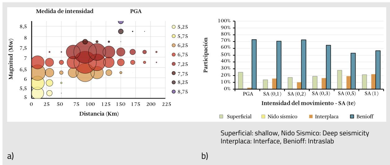
**Figure 6. Disaggregation results for Santiago de Cali city: a) mean PGA with a 10% PoE in 50 years and a combination of magnitude and distance and b) disaggregation by TRT for different intensities measure types.**
