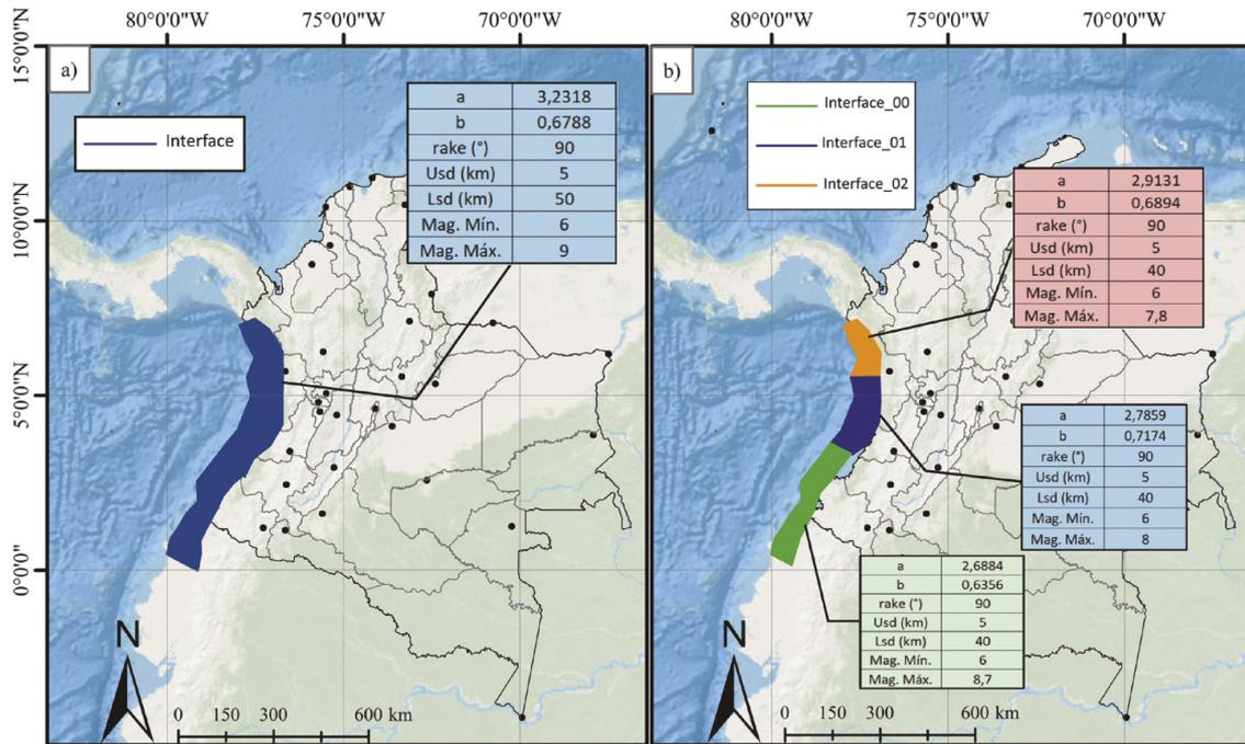
Figure 3. Subduction interface models for Colombia 2018 PSHA study: a) un-segmented model and b) segmented model. The main characteristics of the sources are presented in the tables. Source: Arcila et al. (2020).
