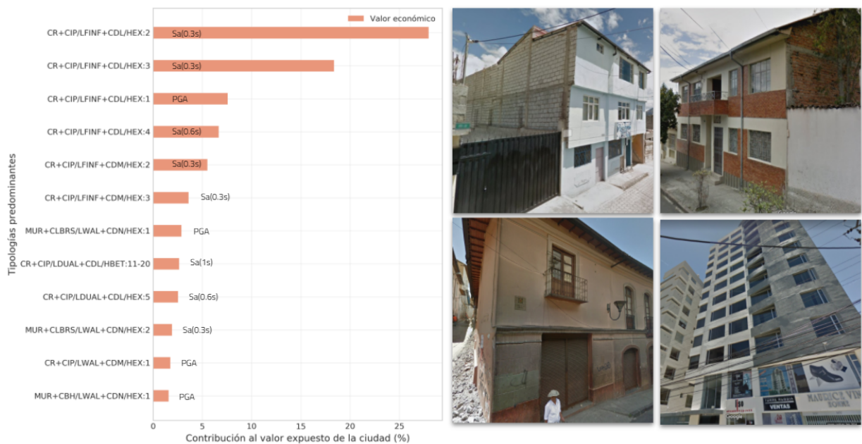
Figure 12. Distribution of exposed economic value in the top 12 building classes in Quito. Over 50% of the value is concentrated in masonry building classes of one to three storeys.
