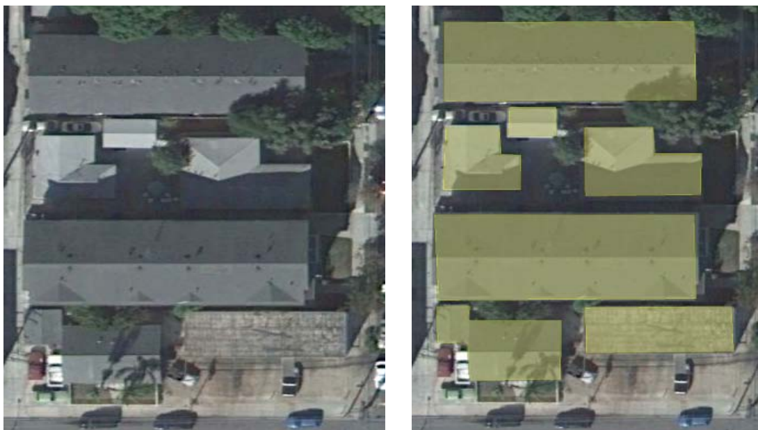
Figure 5.51 Example of building footprint delineation along roofline.
