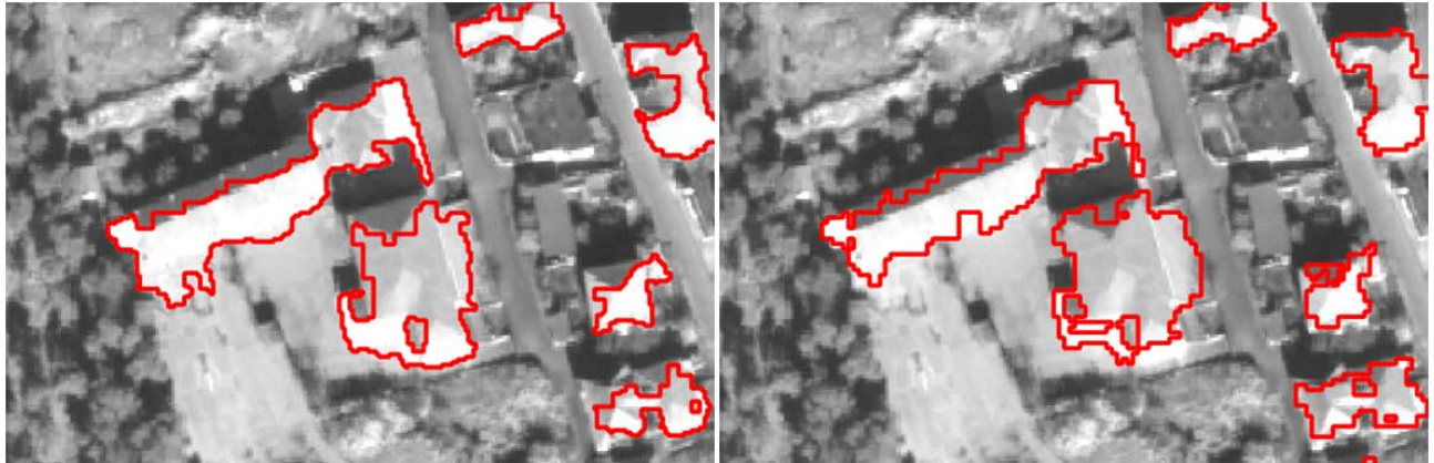
Figure 5.13 Left: Extraction using the unsupervised classification with 9 classes. Right: Extraction using the supervised classification
