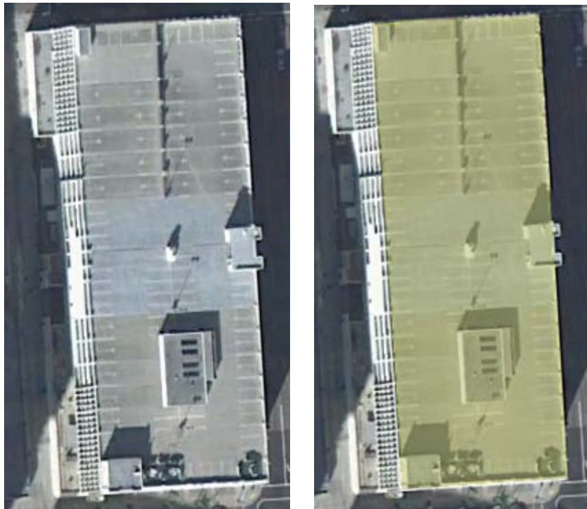
Figure 5.47 Building footprint delineation along roofline.
